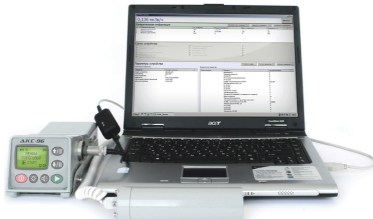
Figure 37. MKS-08 with adapter for transfer data on PC or laptop
